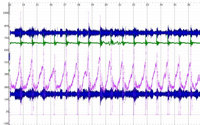
**Fig. 8** Synchronized streams in Sonic Visualizer. Here you can see two channel audio synchronized with accelerometer (top, green) and balanceboard data (bottom, purple).
