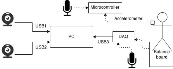
**Fig. 5** Multimodal recording system diagram. Each webcam has a microphone and is connected to the pc via USB. The dashed arrows represent analog signals. The balance board has four analog sensors but these are simplified to one connection in the schematic. The analog output of the microphones is also recorded through the DAQ. An analog accelerometer is connected with a microcontroller which also records audio.
