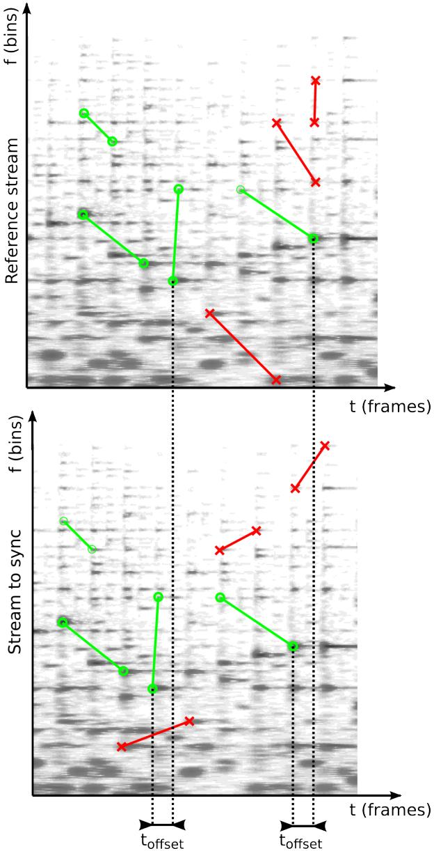
**Fig. 2** Two streams of audio with fingerprints marked. Some fingerprints are present in both streams (green, O) while others are not (red,  $\times$ ). Matching fingerprints have the same offset ( $t_{offset}$ ), indicated by the dotted lines.
