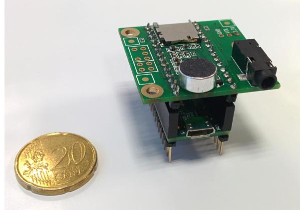
**Fig. 6** A microcontroller fitted with an electret microphone and a microSD card slot. It can record audio in real-time together with sensor data.
