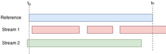
**Fig. 3** A reference stream (blue) can be synchronized with streams one and two. It allows a workflow where streams are started and stopped (red) or start before the reference stream (green).
