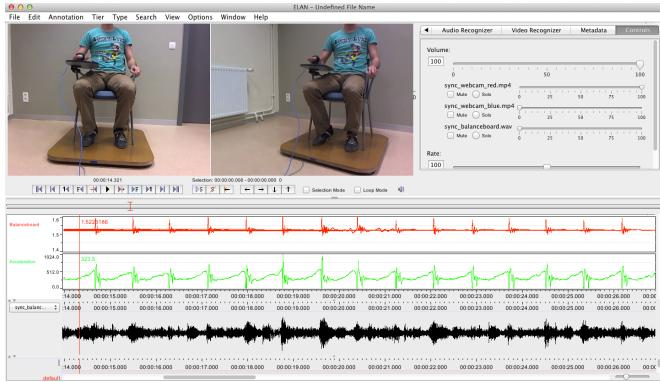
**Fig. 7** The synchronized data from the two webcams, accelerometer and balanceboard in ELAN. From top to bottom the synchronized streams are two video-streams, balance-board data (red), accelerometer-data (green) and audio (black).
