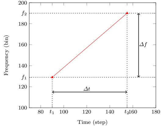
**Fig. 1** A fingerprint consists of two peaks in a time-frequency representation .
