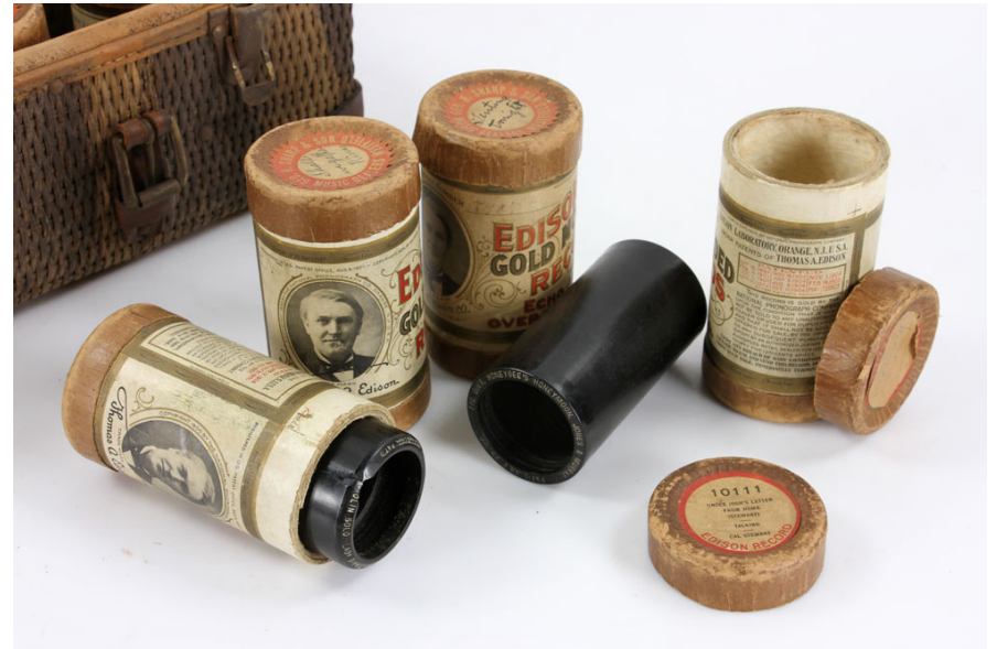
Fig: Wax Cylinders, most popular around 1896–1916 with a capacity of about 2 minutes.
