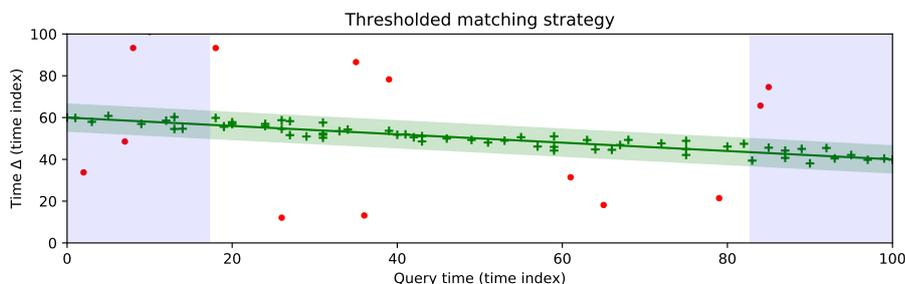
Fig. 7: To discriminate true from false positives a thresholded matching strategy is used. The first few and last few matches (blue background) are used to calculate a median  $\Delta t$ . Accepted matches (green background) fall in a small range around a linear regression from the first to last median  $\Delta t$ . Some random matches (red dots) are dismissed.
