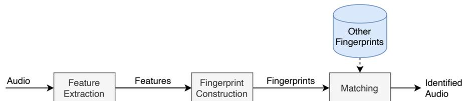
Fig. 5: General acoustic fingerprinting system.
