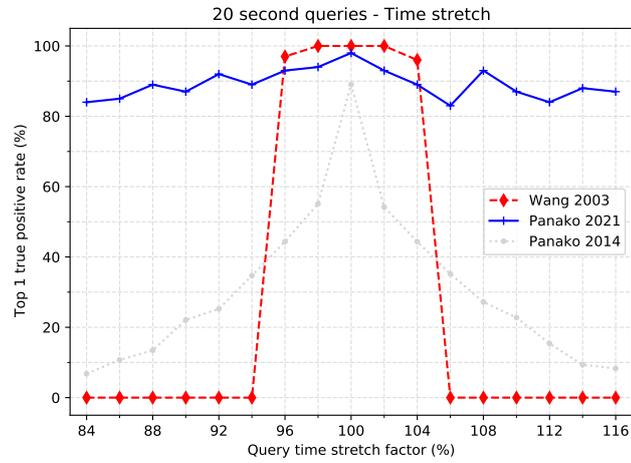
Fig. 10: Comparison of the top one true positive rate after time-stretching for 20s query fragments for Wang 2003 [29], Panako 2014 [23] and Panako 2021.
