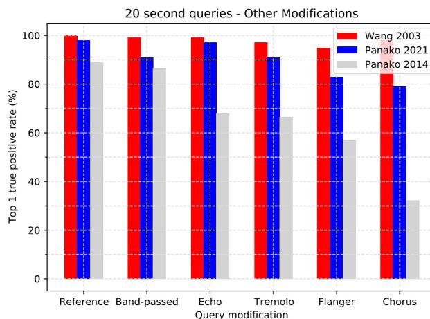
Fig. 8: Comparison of the top one true positive rate after several modifications for 20 second query fragments for Wang 2003 [29], Panako 2014 [23] and Panako 2021.
