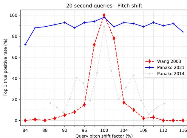
Fig. 9: Comparison of the top one true positive rate after pitch-shifting for 20s query fragments for Wang 2003 [29], Panako 2014 [23] and Panako 2021.
