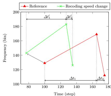
Fig. 6: The effect of speed modification on a fingerprint. The figure shows a single fingerprint extracted from reference audio ( $\blacktriangle$ ) and the same fingerprint extracted from audio after recording speed modification ( $\blackcross$ ).
